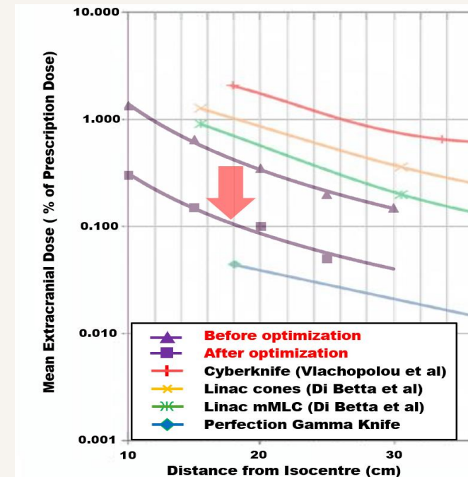
Fig.3 Comparison of Extracranial Doses for Different Radiosurgery units [1] with our improvement for Linac SRS (using MLC)
